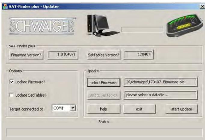
Under <Target connected to..> select the COM-port on your PC (1 or 2) that the SAT-Finder plus is connected to.
