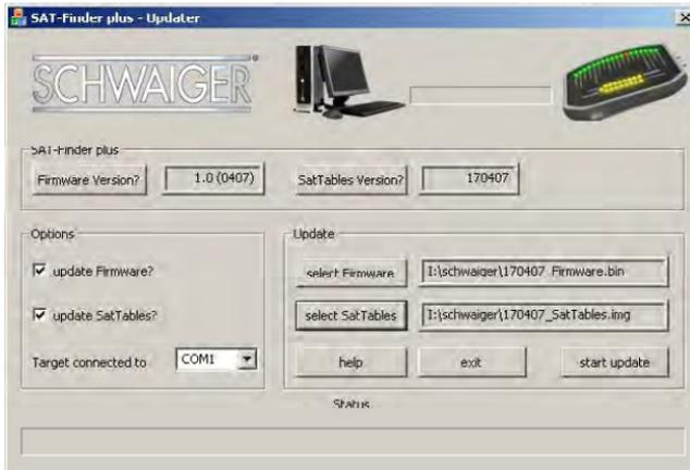
Once the SAT-Finder plus has been recognised and is in update mode, the transfer of the selected file will begin. The status message will change to "transmitting image..." and the progress of the transfer is shown in the status bar.
