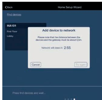
**When registering the LED lamps, ensure that the distance of 0.5m between the Gateway and the LED lamps is not exceeded.**
